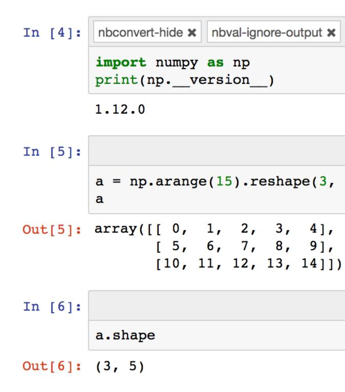
Cell tags are a lightweight way to customise the behaviour of tools working with notebooks; we're working on building support for them into tools like nbconvert and nbval. To start using tags, select Tags in the View > Cell Toolbar menu in a notebook.
